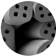
Antron® type 6,6 nylon hollow filament with DuraTech® soil resistance treatment
