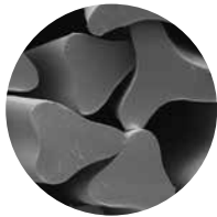
A competitive type 6,6 nylon trilobal with a generic soil resistance treatment
