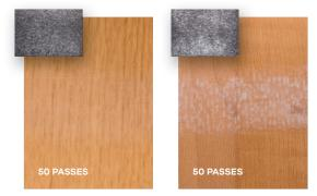
Our proprietary blend of aluminum oxide particles is suspended evenly through the urethane top coat, giving the industry's best abrasion resistance. (Results after 50 passes with sanding block.)
