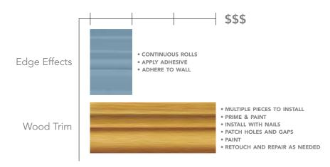
Edge Effects is more economical than traditional wood trim. Available in continuous rolls saving installation time and money. And once installed, it has lower maintenance costs than natural wood bases. Over time, Edge Effects offers the best lifecycle value.
