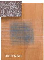
With new protective compounds from the aerospace industry and dentistry, Quantum Guard Elite's stain resistance performs over time at the same high level as the day it was installed. (Results after 1,000 passes with a sanding block, staining with a blue Sharpie and cleaning with an alcohol wipe.)
