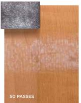
Our proprietary blend of aluminum oxide particles is suspended evenly through the urethane top coat, giving the industry's best abrasion resistance. (Results after 50 passes with sanding block.)
